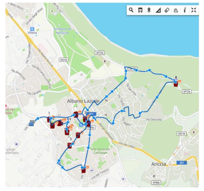
Figure 19. Collection route of 19 containers with distance optimization.
