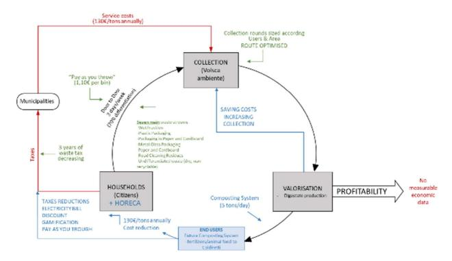
Figure 23. Flow chart of the system to be implemented for the recovery of OFMSW from households and HORECA in Albano Laziale.
